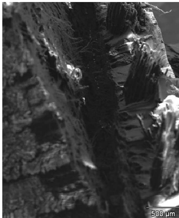
Figure 7 SEM micrograph showing the fracture surface of a JPJ specimen failed in flexure.
